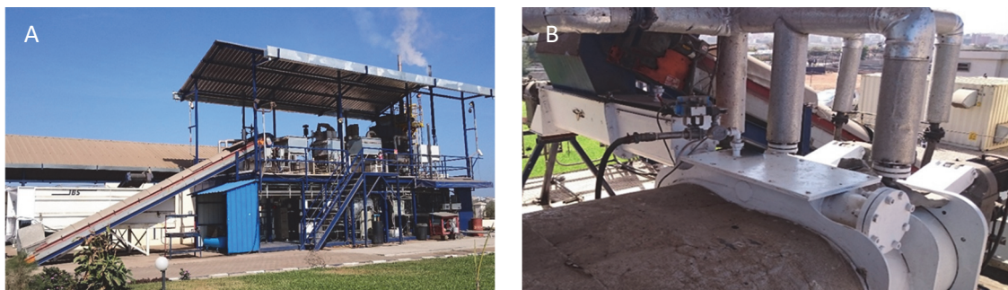
Figure 4.16 A) a contact dryer at the Omni-processor pilot plant at Niayes FSTP in Dakar, Senegal. In this plant, the sludge is incinerated leading to the generation of heat and electricity. B) part of the heat from combustion is recirculated in the process for the drying of the sludge with this contact dryer unit (photos: UKZN PRG).
