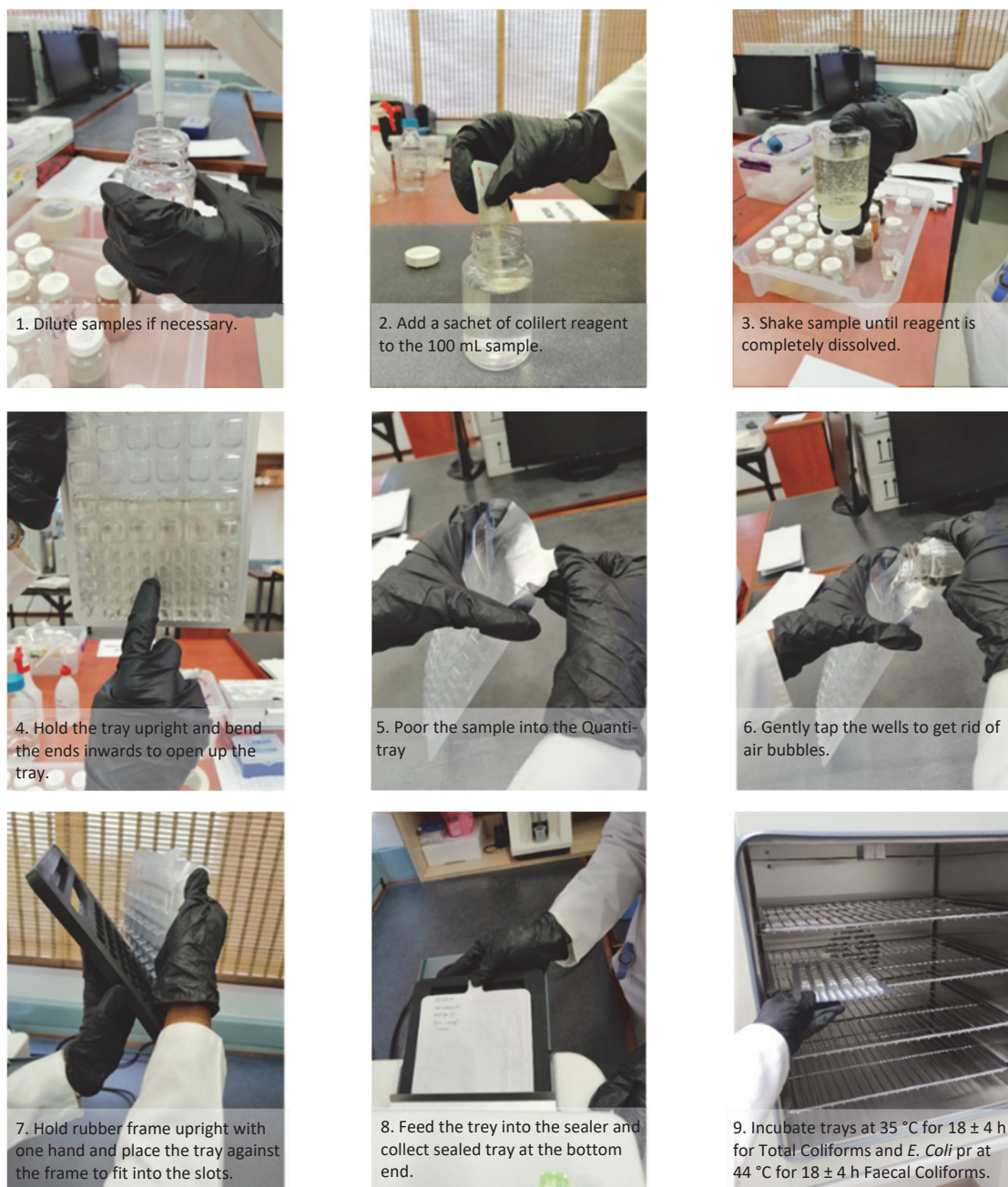
Figure 8.21 Quanti-Tray 200 total coliforms and E. coli procedure (source: UKZN PRG).
