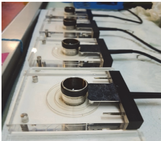
Figure 4.7 Example of replicates being measured in a CST test to determine sludge dewatering time (photo: Eawag).
