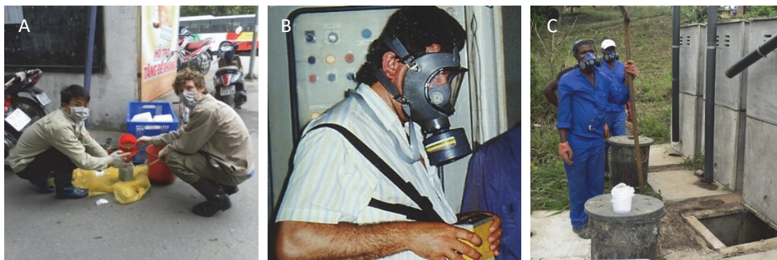
Figure 3.22 Personal protective equipment. A) transferring homogenised samples to sample containers with a plastic funnel and ground protection. B) a mask and meter/alarm for H_2S . C) collecting samples from pit latrines (photos: Eawag, M. Henze, UKZN PRG, respectively).
