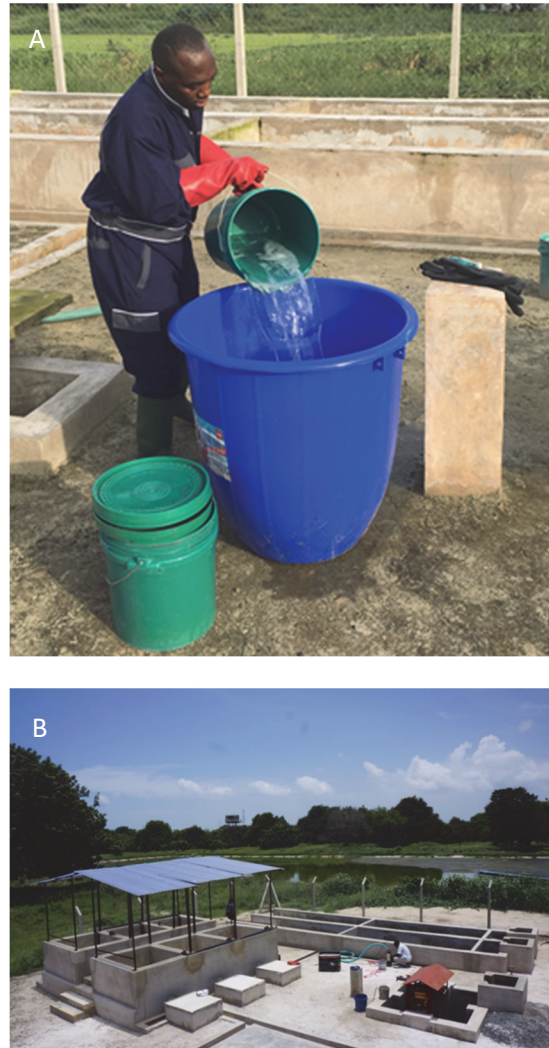
Figure 4.9 A) mixing chitosan conditioner for pilot-scale trials. B) the pilot-scale dewatering research facility at the University of Dar es Salaam, including the settling-thickening tanks, conditioner mixing tank, and six sand drying beds (photos: Eawag).
